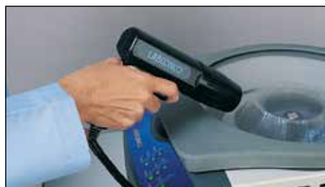
CentriZap Strobe Light allows the user to check sample status without stopping the rotor and opening the lid.
