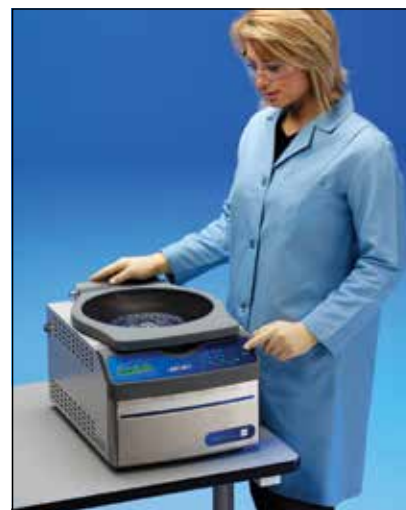
CentriVap Vacuum Concentrators, such as the Acid-Resistant CentriVap shown above, process up to 132 samples at once.
