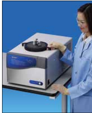
CentriVap -50 Cold Trap, which reaches -50° C (-58° F), collects moisture during evaporation to protect the vacuum pump.
