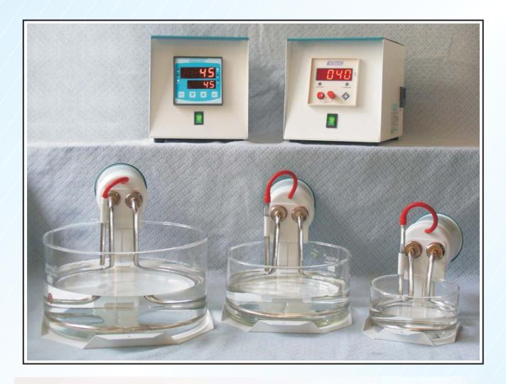
**EQUITRON** Glass Oil Baths are ideal for small scale research and development reactions as well as for tempering applications in laboratories.
